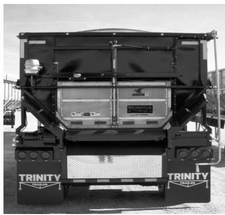
Figure 96 - Hydraulic Lift Top-Hinge With Hydraulic Slide-Up Door
