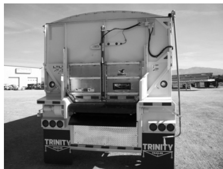
Figure 92 - Full Swing With Hydraulic Slide-Up Door
