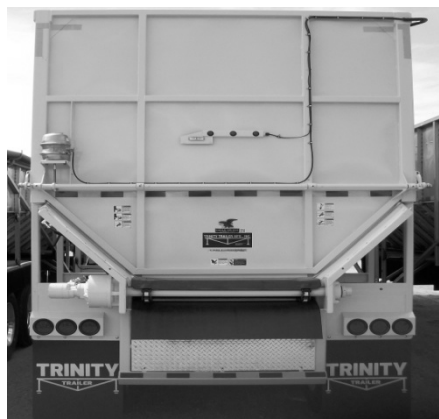
Figure 94 - Hydraulic Lift Top- Hinge With No Lower Door
