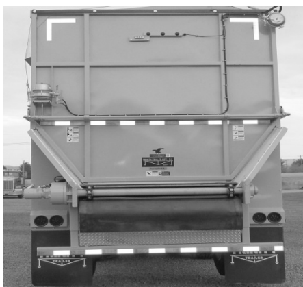
Figure 93 - Pneumatic Lift Top- Hinge With No Lower Door
