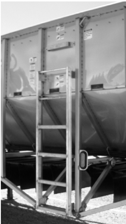
Figure 153 - Roadside Ladder Showing Offset
