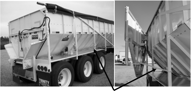
Figure 100 - Full-Swing Door Latch Components
