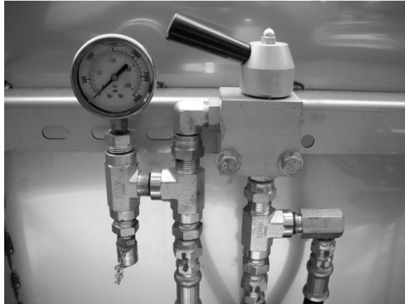
Figure 110 - Needle Valve Used to Control Conveyor Speed with Electric or Gas Driven Hydraulic Systems
