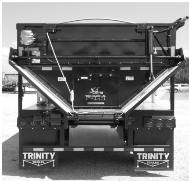
Figure 97 - Hydraulic Lift Top-Hinge "Spud" With Hydraulic Flip-Up Door
