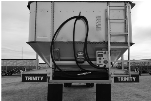
Figure 132 -Pneumatically-Actuated Front Wet Seal
