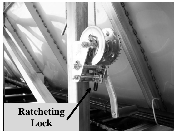
Figure 127- Fold-Down Sideboard Door Operator Winch
