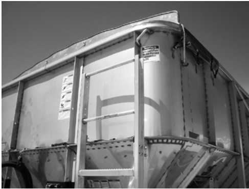
Figure 151 - Front Ladder Showing Upper User Fall Protection Device
