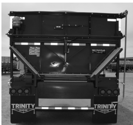
Figure 95 - Hydraulic Lift Top-Hinge with Hydraulic Flip-Up Door
