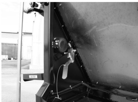
Figure 106- Slide-Up Door Clamp Latch Disengaged
