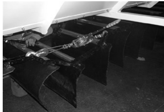
Figure 6 - Using Come-Along To Pull Up Chain Slack
