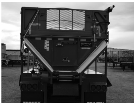
Figure 89 - Full Swing "Spud" With Hydraulic Flip-Up Door
