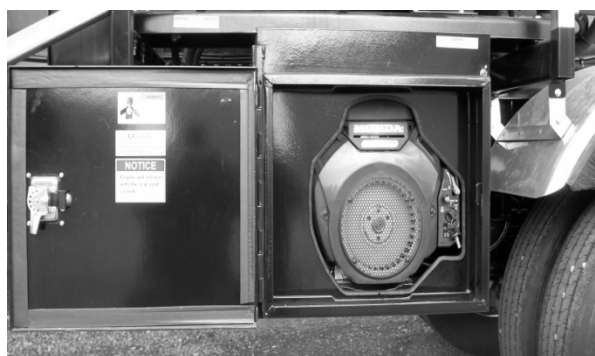
Figure 107 - 20 HP Gas Engine (Shown in Optional Enclosure)
