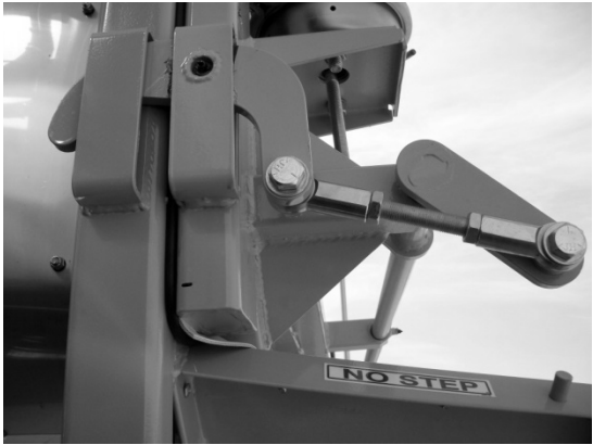
Figure 104 - Top Hinge Pneumatic Latch Disengaged
