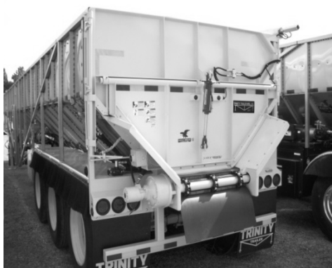
Figure 91 - Full Swing With Hydraulic Flip-Up Door
