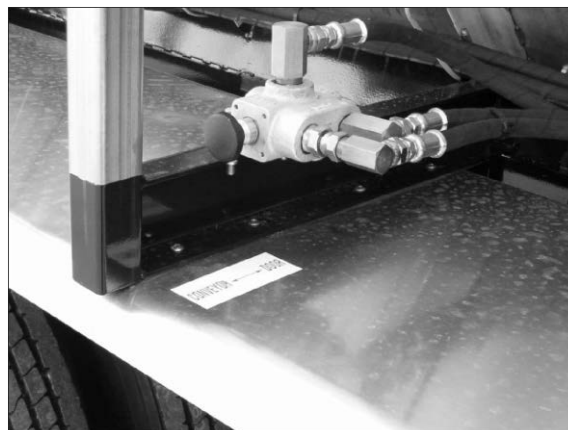
Figure 112 - Push-Pull Valve Used to Select Door or Conveyor
