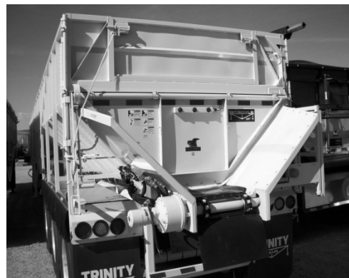
Figure 88 - Full Swing "Spud" With Manual Flip-Up Door
