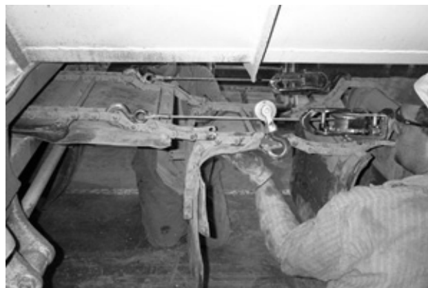
Figure 7 - Determine How Much Chain To Remove
